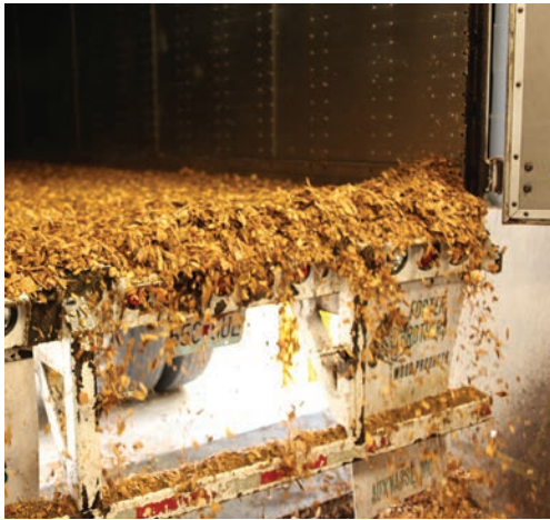
Wood residues are unloaded into the biomass receiving hopper.
