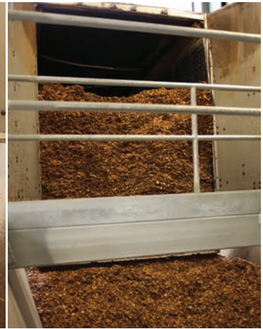
A drag conveyor delivers wood residues to storage silos.
